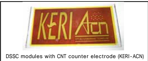
CNT Counter Electrode of DSSC
